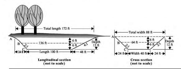
As an example, assume a pond with a depth, D, of 12 feet, a bottom width, W, of 40 feet, and a bottom length, L, of 100 feet as shown in figure 35. The side slope at the ramp end is 4:1, and the remaining slopes are 2:1. The volume of excavation, V, is computed as follows:
